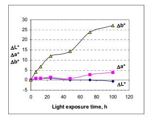
Figure 4. Example of color change with exposure time for a yellow ink jet print.
