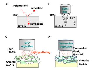
*Figure 5. Light behavior in depth profiling*<sup>7</sup>.
