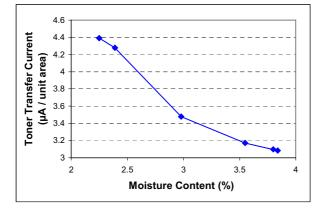
Figure 2. Influence of moisture content of paper on toner transfer current.
