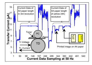
Figure 1. Measurement of transfer current. Sampling at 50 Hz.
